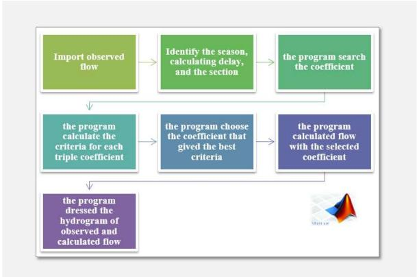
Figure 4. Execution steps of the program under Matlab
